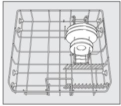
Both sides of the rear section of the spiked insert can be lowered to make more room for large items, e.g. pots, pans and dishes.
